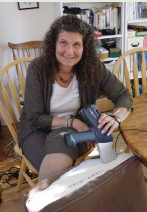
Blum testing for traces of brominated fire retardants in furniture foam with an x-ray fluorescence analyzer.
